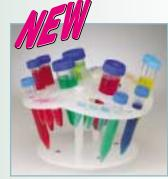
compact holder is designed to be easily secured to the platform of a shaker with included screws. Made from polypropylene and steam autoclavable at  $121^{\circ}C$  (250°F). Dimensions: 15.9cm (6<sup>1</sup>/<sub>4</sub>") base diameter, 21cm (8<sup>1</sup>/<sub>4</sub>") tube holder diameter, 12.7cm (5") height.
